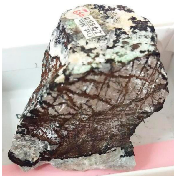
Figure 6. A specimen labelled as domeykite ( \text{Cu}_3\text{As} ; OUNHM MIN.27550), displaying patches of a dark navy-blue efflorescence and lines of a cocoa brown efflorescence, which have likely formed by the off-gassing of storage material or the deterioration of neighbouring specimens. Image used with permission of Oxford University Natural History Museum.
