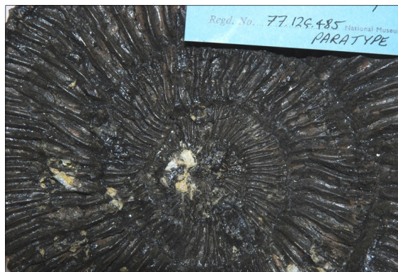
Fig. 2. Damage from pyrite decay to one of the specimens ( Pectinatites reisiformis , NMW 77.12G.485); pyrite decay products are visible as yellow-white powdery substance.
