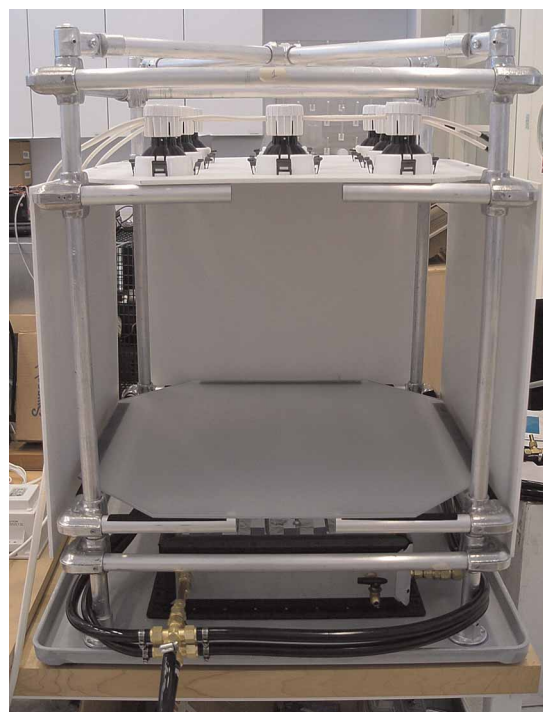
Figure 2 Lighting scaffold positioned above exposure case with diffuser plate and three of four side panels mounted.
