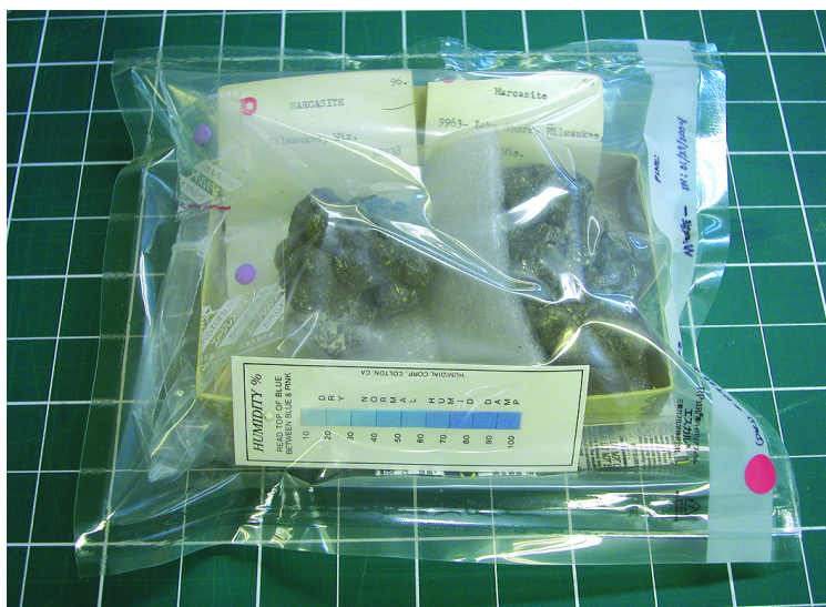
Figure 4. Example of final enclosure of marcasite specimen in the RP System
