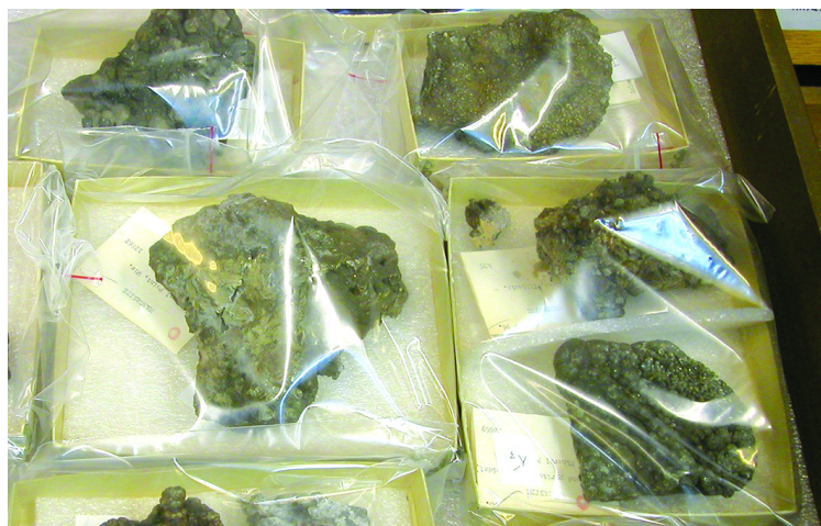
Figure 3. Final preparation of marcasite specimens with polyethylene bags
