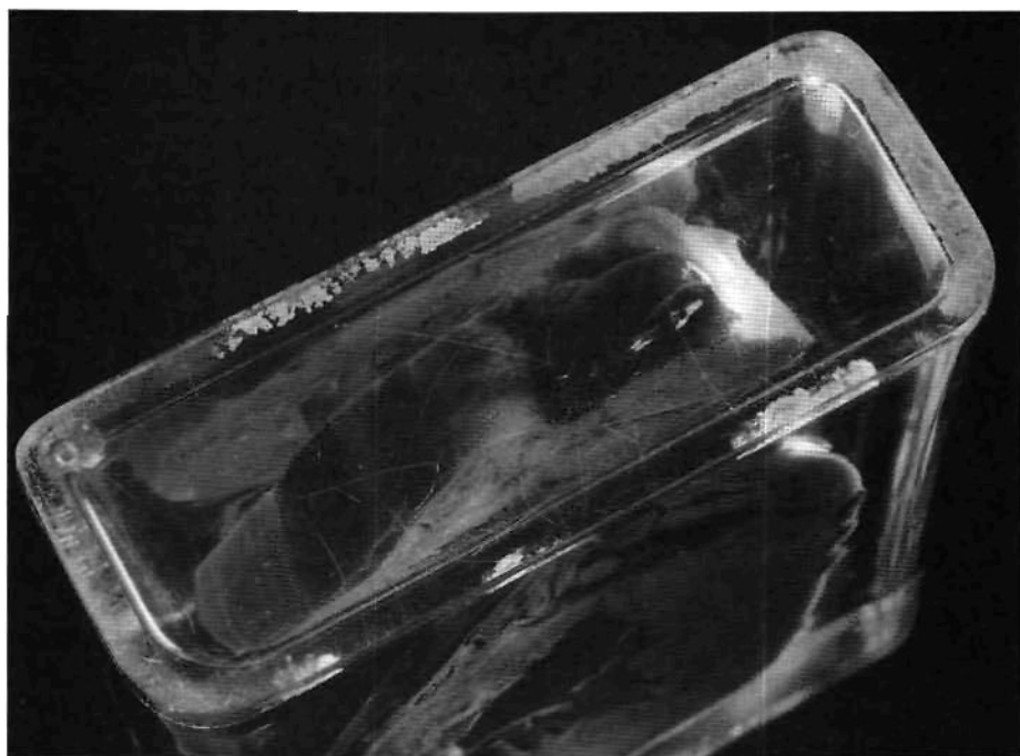
Figure 2. Partially split seam of a Plexiglas ® jar.
